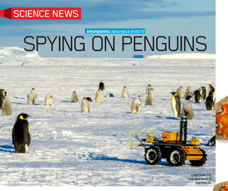
Meet ECHO: A four-wheeled robot helping scientists monitor Emperor penguins in Antarctica. The autonomous vehicle can independently navigate the vast, frozen terrain. ECHO is equipped with a 360-degree camera and sensors to spot penguins, as well as an antenna to detect whether any of the birds have been tagged with a tracking chip.
